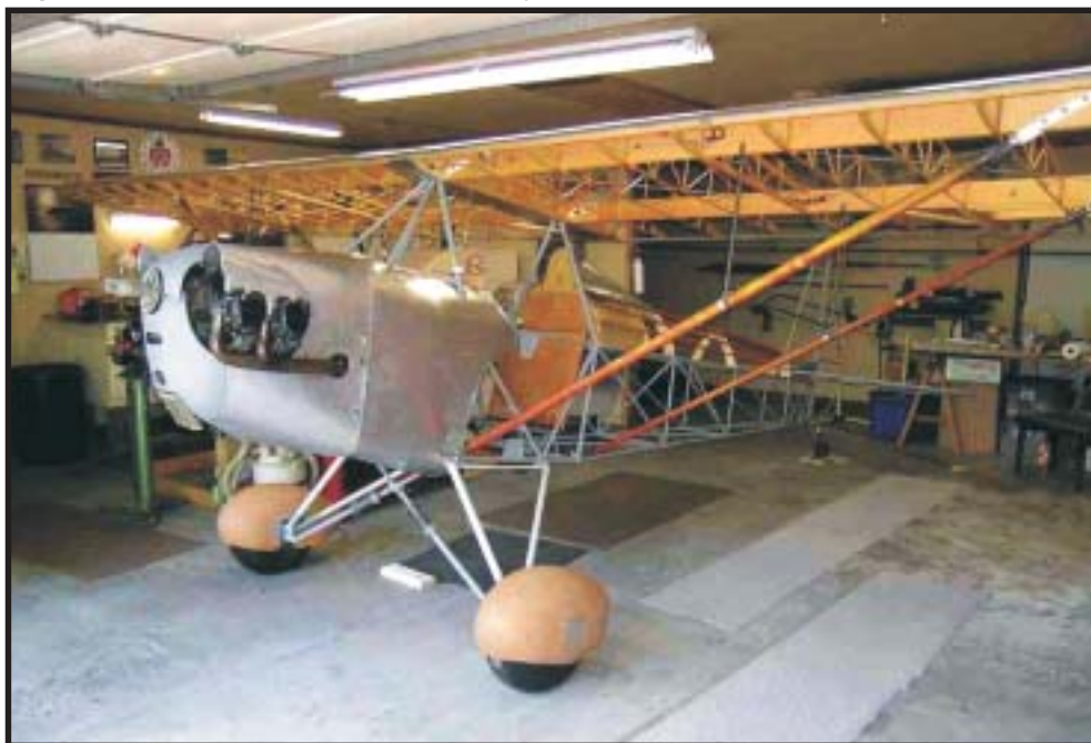
"Scratch built" means that Steve McGuire has built every piece of his Baby Ace. No kit parts here! Steve learned how to weld and is doing the job one piece at time.
