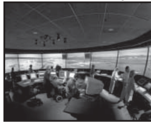
Interior view- note the 360-degree computer-simulated visual display.
