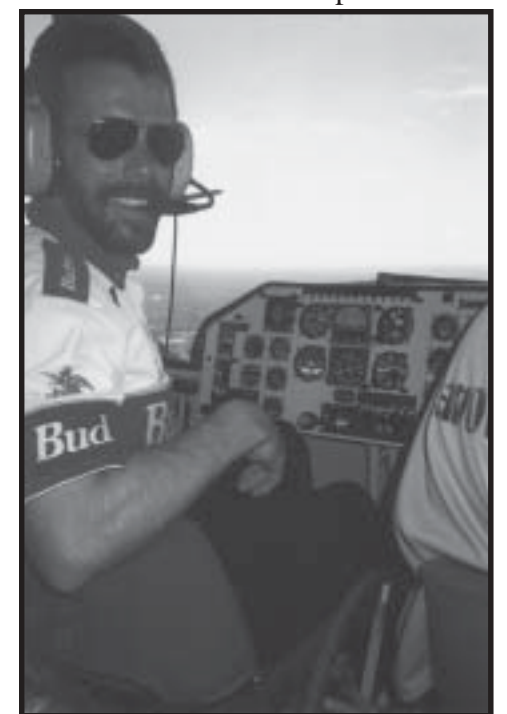
Chief Pilot Carl Harbuck, 3500 flight hours in the airship and a very pleasant guy. Note the IFR panel and the pitch control wheel between the seats. Lateral control is via rudder pedals.
