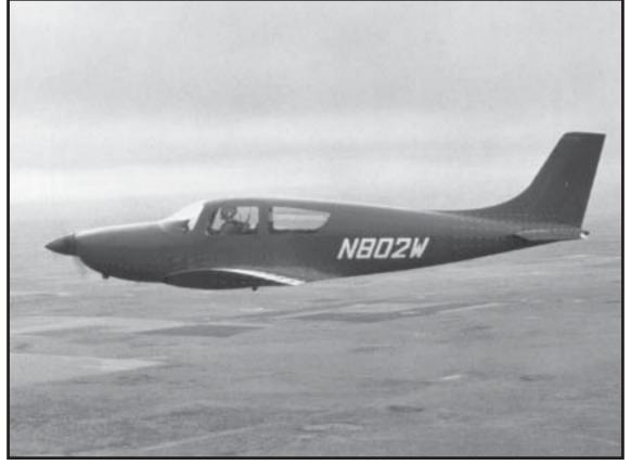
The Windecker Eagle N802W during certification flight testing, with test pilot Bill Robinson at the controls Note the tufting on the wing root and empennage. In contrast with the pre-production airplane, this one had retractable gear.
