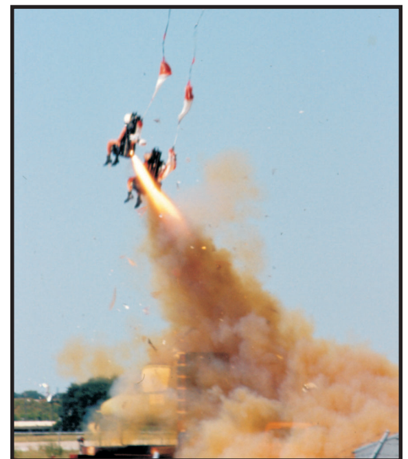
The XV-15 ejection seats firing on the ramp at TUL. Photo by Ken Cook, a Rockwell engineer, using a handheld camera. Ken is retired near Lake Tenkiller and recently finished a beautiful Vans RV-4.
